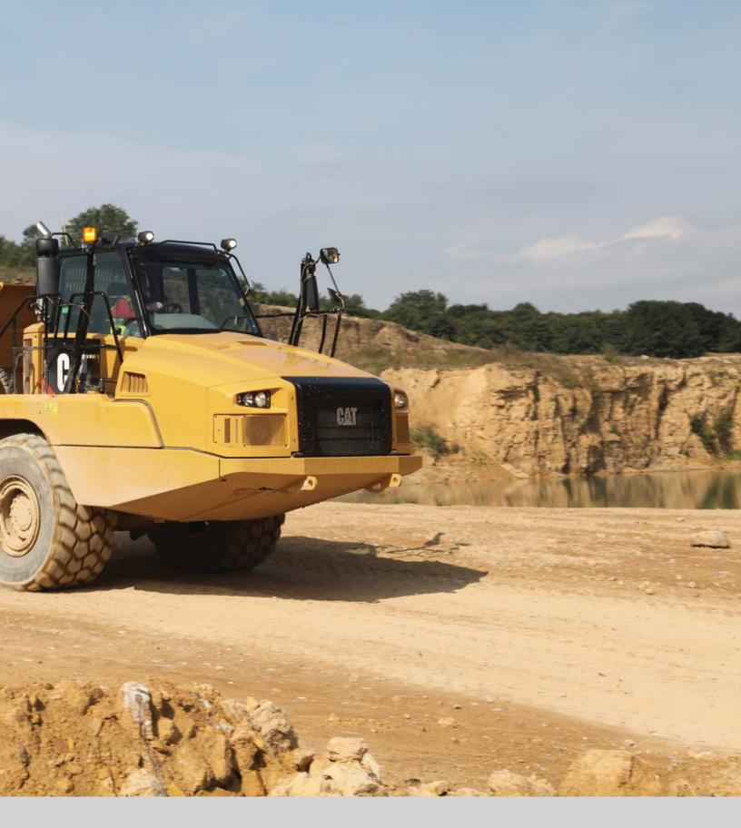
Strong, durable Cat C9.3 ACERT engine platform with U.S. EPA Tier 4 Final/EU Stage IV engine emission solution.
